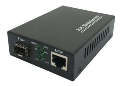
The PoE media converter can provide both Ethernet data and power over RJ45 cable, it can be used as Ethernet Power Sourcing Equipment and automatically detect and identify connected devices, such as IP cameras which comply with standard IEEE PoE 802.3af, 802.3at, and then supply power for them. The PoE media converter makes easier the deployment of Wireless AP, IP camera and IP-based Network equipment.
